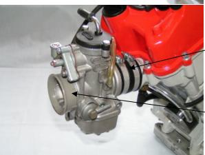
Put the carburetor into the carburetor rubber and tighten both hose clamps.
