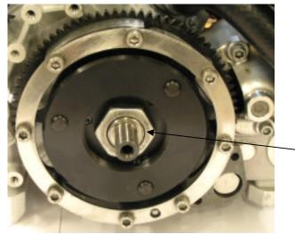
Install the clutch onto the crankshaft (do not forget the key).
