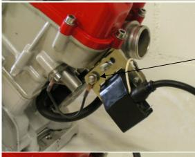
Put the ground cable onto the stud of the lower silent block.
