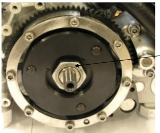
Loosen the clutch mount nut.
