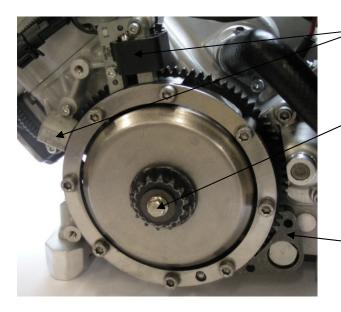
Dismantle the primary coil and the pick-up sensor.
