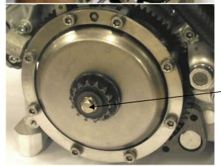
Install the clutch drum and the transmission sprocket bearing. Mount the "BATMAN"-tool.
